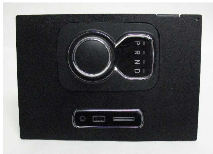
Fig 8 - Rotary Gear Shifter and USB/AUX/SD Card Module in Faceplate
