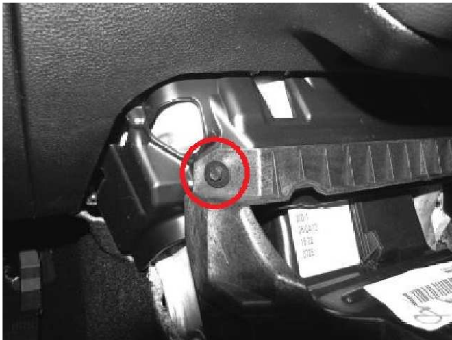
Fig 3 - Front Sub Structure Screws
