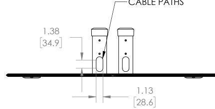
WEIGHT CAPACITY: 160 LBS DIMENSIONS ARE IN INCHES AND [MM]
