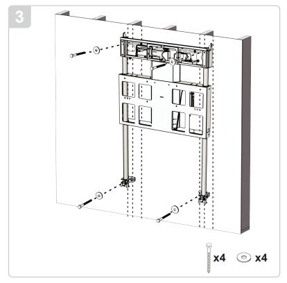
Step 3: With a minimum of two people raise the FPS-200 and secure it to the wall with the 5/16" x 3" lag bolts and flat washers. Note: If you plan to toggle the bolts to steel studs in either the top or bottom mounting points, the 1/4" pilot hole will have to be drilled out with a 5/16" drill to allow for the wedge anchors to be a minimum depth of 3" (75mm).
