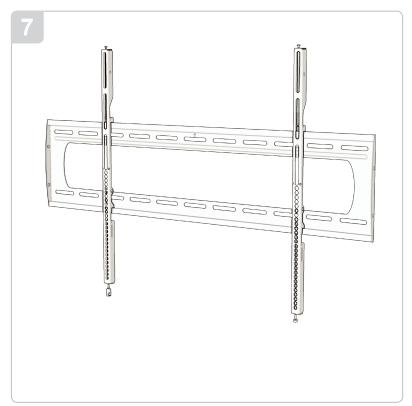
Step 7: Install the "P" series flat mount with the supplied hardware, following the installation instructions supplied with the "P" series flat wall mount. Make sure you center the mount to conform with the original center travel height that you previously marked on the wall.
