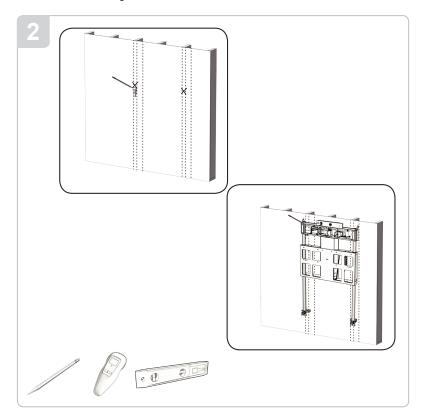
Step 2: With a stud finder, locate the 16" or 24" mark on the center studs inside the wall closest to the desired mounting point and center the mount left to right, then top to bottom. With your pencil, mark the upper and lower left and right mounting points through the mounting plate. Set the FPS-200 aside and drill the four pilot holes.
